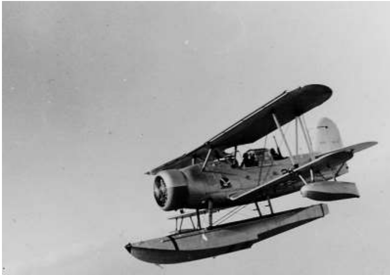
Curtiss SOC-3 scout observation floatplane similar to those carried aboard the Savannah (CL-42). Note the .30-cal. machine gun in the after cockpit. U.S. Naval History and Heritage Command photograph #NH 80523
