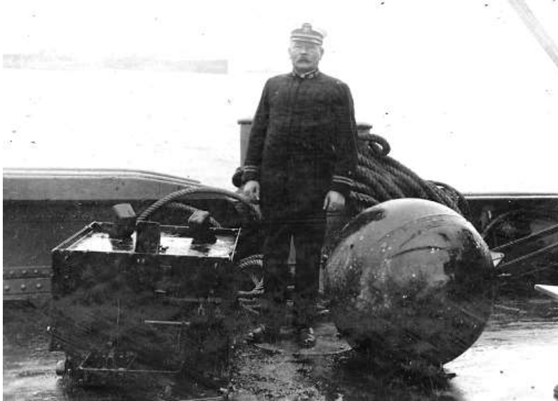
An American Mk VI mine, complete with anchor, recovered in the North Sea. Naval History and Heritage Command photograph #NH 2507
