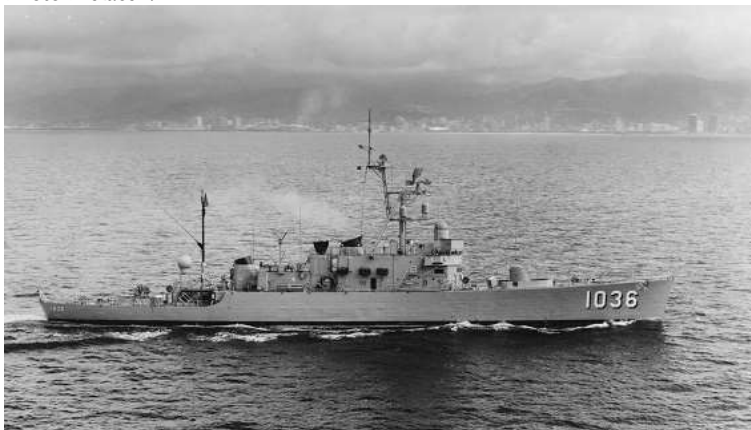
Destroyer escort USS McMorris (DE-1036) off Oahu, Hawaii, 10 March 1972; she is displaying “Spooky” electronics arrays fitted in this class of DE. Naval History and Heritage Command photograph #NH 82940
