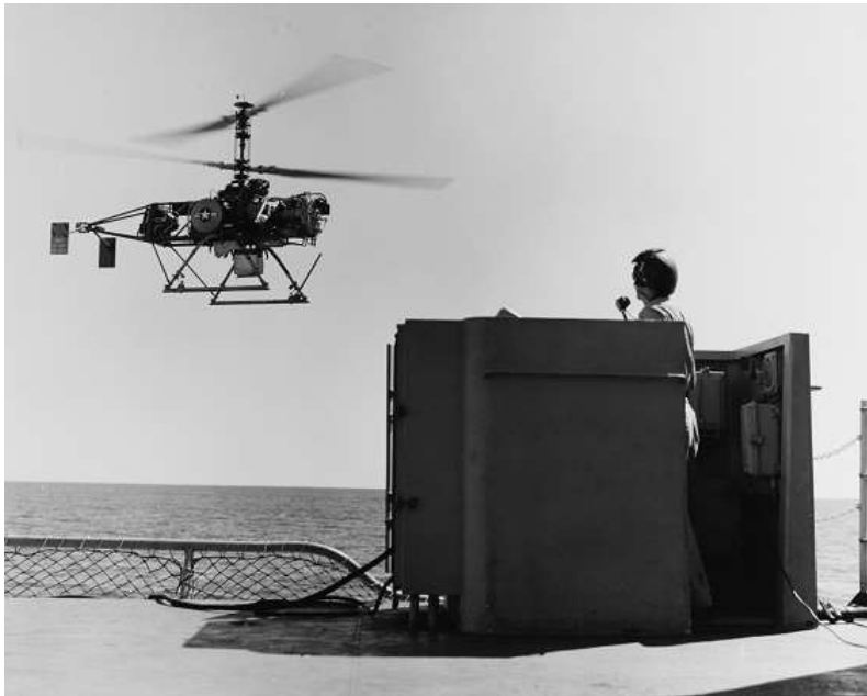
A drone anti-submarine helicopter (DASH) under the control of Lt. (jg) Mark S. Barg, aboard the USS Nicholas (DD-449), off the coast of Oahu, Hawaii, 10 February 1965. National Archives photograph #USN 1111342
